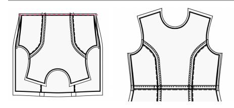
9. Place the right Back Bodice and right Back Skirt together with right sides together, matching the side seams. Pin the bodice to the skirt, matching the darts/notches. Consider basting the seam first to be sure the seams match up perfectly and to prevent any shifting of fabric when stitching. Stitch together. Serge the seam allowances, and press them towards top. Repeat for the left Back Bodice and Left Back Skirt. Treat as whole Back pieces in the future.
