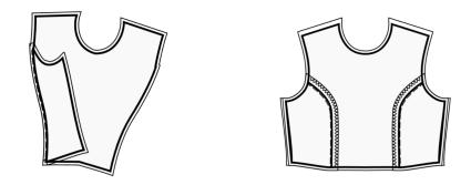
6. Sew darts on Back pieces. Start from the edge of the fabric, and stitch towards the dart corner, using a narrow stitch. Do not backstitch, leave long threads and tie a knot. Press bulk of darts towards center back (see Figure in the right).
