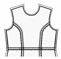
9. Place the right Back Bodice and right Back Skirt together with right sides together, matching the side seams. Pin the bodice to the skirt, matching the darts/notches. Consider basting the seam first to be sure the seams match up perfectly and to prevent any shifting of fabric when stitching. Stitch together. Serge the seam allowances, and press them towards top. Repeat for the left Back Bodice and Left Back Skirt. Treat as whole Back pieces in the future.
