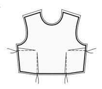
5. Sew darts on Back pieces. Start from the edge of the fabric, and stitch towards the dart corner, using a narrow stitch. Do not backstitch, leave long threads and tie a knot. Press bulk of darts towards center back (see Figure in the right).
