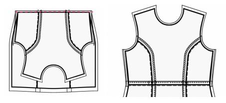
9. Place the right Back Bodice and right Back Skirt together with right sides together, matching the side seams. Pin the bodice to the skirt, matching the darts/notches. Consider basting the seam first to be sure the seams match up perfectly and to prevent any shifting of fabric when stitching. Stitch together. Serge the seam allowances, and press them towards top. Repeat for the left Back Bodice and Left Back Skirt. Treat as whole Back pieces in the future.
