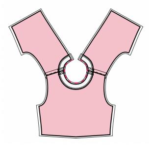
13. Cut (or take ready) bias tape, its width should equal 3 cm and its length should equal 7 cm. Fold tape in half lengthwise and stitch at 0.3 from edge. Trim seam allowances and turn the piece right side out. Cut 2 loop buttonholes.
