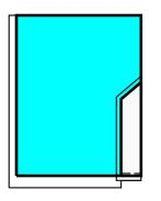
15. Serge the straight area along the lower edge of the sleeve, between the dashed lines. Turn under, press and topstitch or slip stitch as desired. Make and baste the pleats according to the dashed lines and to the technical drawing. Slipstitch 3-4 cm along the inner fold at the sleeve cap.
