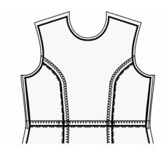
9. Place the right Back Bodice and right Back Skirt together with right sides together, matching the side seams.
