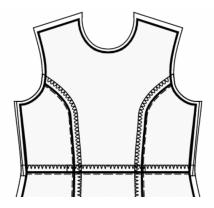
9. Place the right Back Bodice and right Back Skirt together with right sides together, matching the side seams.
