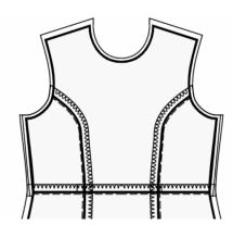
11. Place the right Back Bodice and right Back Skirt together with right sides together, matching the side seams. Pin the bodice to the skirt, matching the darts/notches. Consider basting the seam first to be sure the seams match up perfectly and to prevent any shifting of fabric when stitching. Stitch together. Serge the seam allowances, and press them towards top. Repeat for the left Back Bodice and Left Back Skirt. Treat as whole Back pieces in the future.
