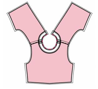
8. Apply fusible interfacing to the area of button placket (one-piece with front).
