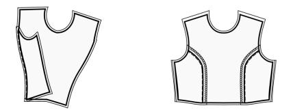
7. Sew waist darts on Back pieces if these are present on your sewing pattern. Start from the edge of the fabric, and stitch towards the dart corner, using a narrow stitch. Do not backstitch, leave long threads and tie a knot. Press bulk of darts towards center back (see Figure in the right).
