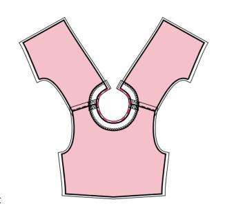
10. Slash slit on sleeve along the marked line. Stop at 1 cm from the end. (Figure 1)
