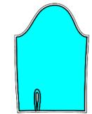
13. Serge the straight area along the lower edge of the sleeve, between the dashed lines. Turn under, press and topstitch or slip stitch as desired. Make and baste the pleats according to the dashed lines and to the technical drawing. Slipstitch 3-4 cm along the inner fold at the sleeve cap.
