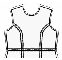
7. Place the right Back Bodice and right Back Skirt together with right sides together, matching the side seams. Pin the bodice to the skirt, matching the darts/notches. Consider basting the seam first to be sure the seams match up perfectly and to prevent any shifting of fabric when stitching. Stitch together. Serge the seam allowances, and press them towards top. Repeat for the left Back Bodice and Left Back Skirt. Treat as whole Back pieces in the future.
