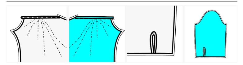
7. Serge the straight area along the lower edge of the sleeve, between the dashed lines. Turn under, press and topstitch or slip stitch as desired. Make and baste the pleats according to the dashed lines and to the technical drawing. Slipstitch 3-4 cm along the inner fold at the sleeve cap.
