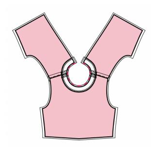
6. Make and topstitch tucks on the sleeve cap. The bulk of the tuck should be on the right side. Use the cardboard control pattern block to verify the shape of the ready cap.
