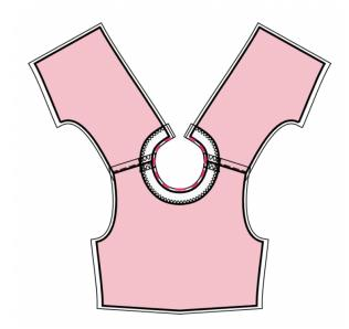
9. Pin collars pairwise right sides together and sew outer edge and corners. Trim seams, turn collar right side out and press.
